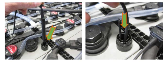
If the probe is correctly inserted and is in contact with the electrolyte, the **SPY-BATT** turns off the "Level" led showing the following display:
