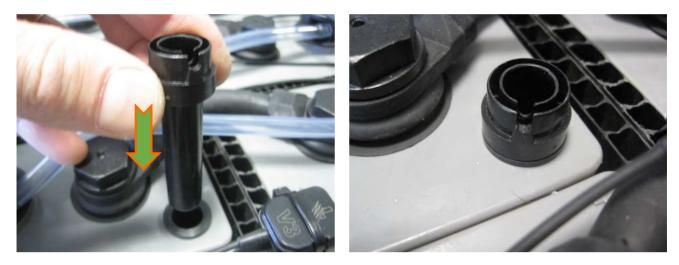
Insert the wired probe bulb into the cylinder and pushing until it stops:
